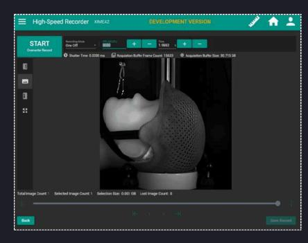
Recording images directly into the memory minimizes transfer delays and enables to user to directly selected only the interesting parts of the record.
