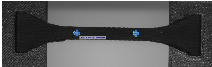
▲ Figure 3: Line Probe placement on the gauge length
