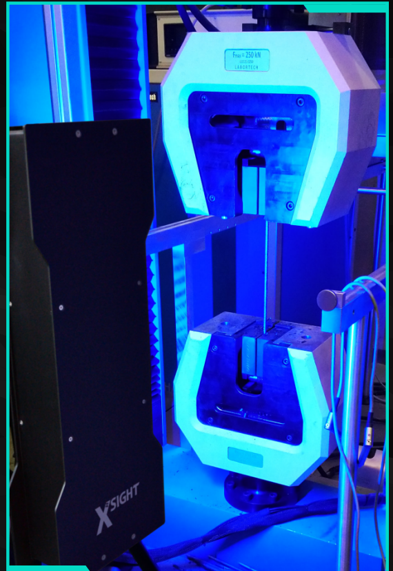
Tensile test set-up for reinforcing steel bars with the ROD measuring system
