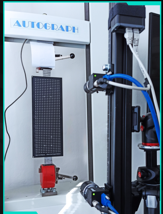
Tensile test set-up shown during the calibration process
