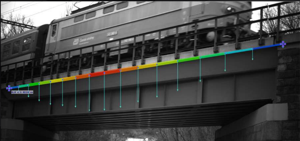
The visualization of deflections [mm]
