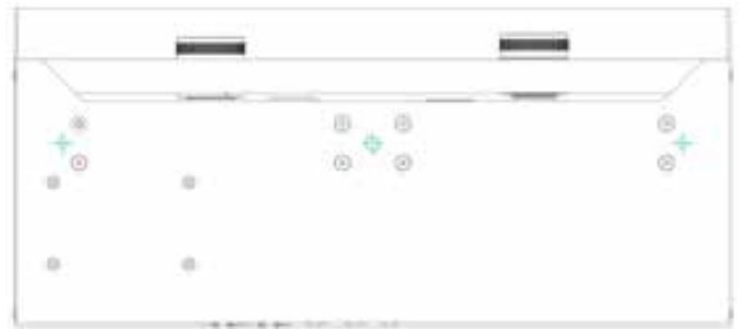
▲ The bottom plate of the ONE LARGE D - 3/8" UNC in the middle and M6 screw holes
