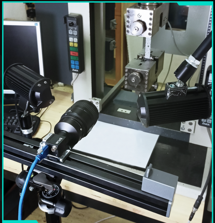
Test setup for notched sample under tensile load
